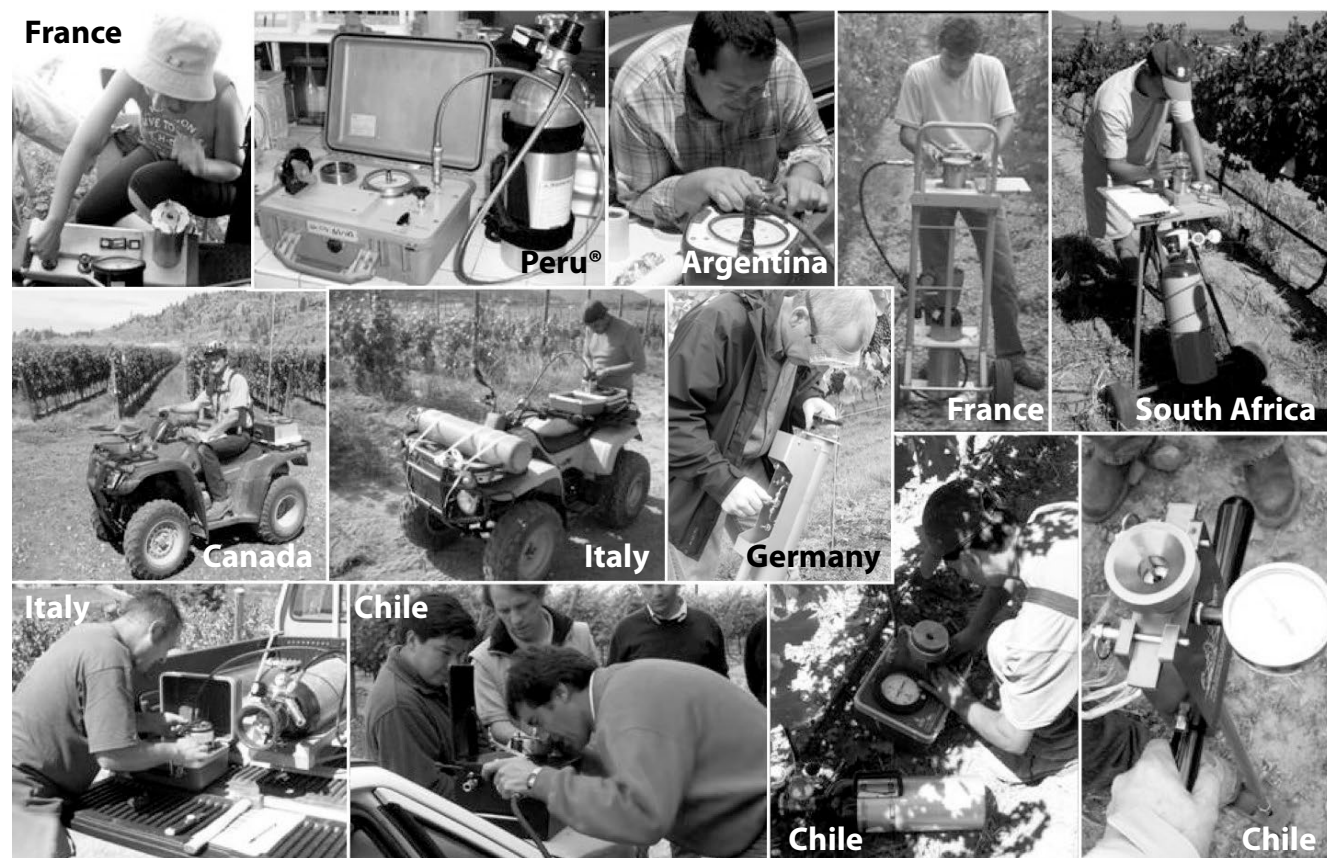
FIGURE 4. Determining vine water status with the pressure chamber
