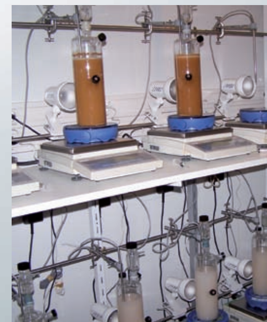
To assess the fermentation performance of the different Lallemand yeast strains and the efficiency of nutrients, a system for online monitoring of fermentation has been developed in close collaboration with INRA Montpellier (thanks to the expertise of the Team UMR-SPO).
